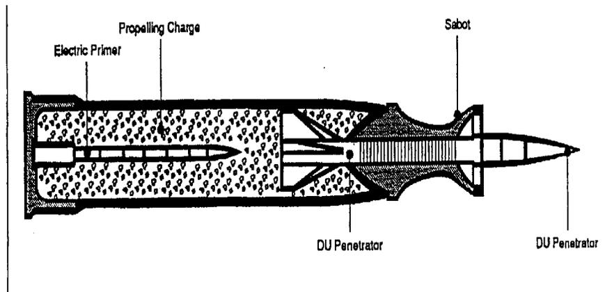
**Figure 1:** Schematic diagram of 120-mm DU penetrator. Source: *Operation Desert Storm: Army Not Adequately Prepared To Deal With Depleted Uranium Contamination*, U.S. General Accounting Office Report, GAO-NSIAD-93-90 (1993), p. 13.
